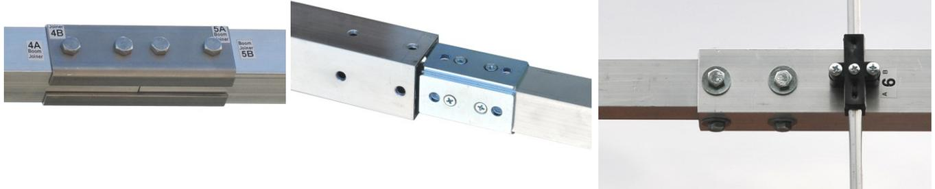
Put the boom on the flat surface. Because of length you should tighten screws lightly for the first moment. Then look along the boom to see if any distortion occurs. When you are satisfied tighten firmly. Before tightening all screws, apply thread lock like Loctite 243 or Permatex Threadlocker BLUE.
