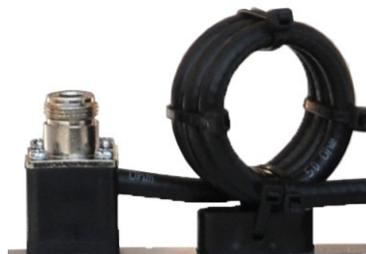
Screw connector to connector holder
