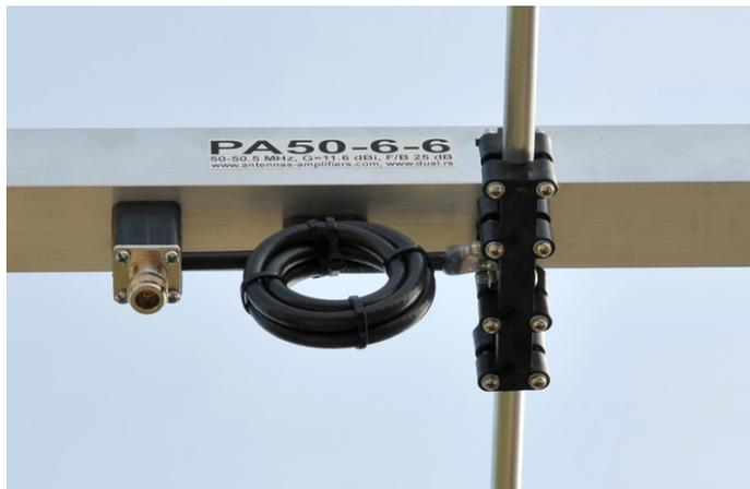
If needed align elements and screw tightly. Elements must stand in one plane.
