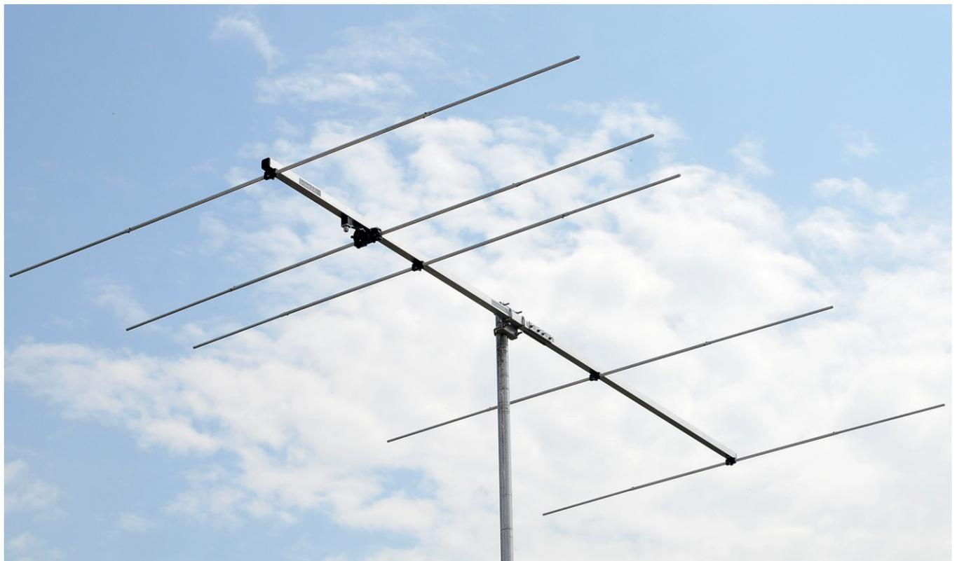
Raise the antenna. Measure SWR. It must be as predicted or very close on all frequencies. Low SWR is a sign that you assembled everything correctly. Best DX - EME.
