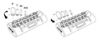
NOTE: Ensure that the batteries are pressed down all the way to ensure optimal contact.
