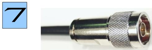
The prepared cable tail has to be inserted into the housing until stop. Tighten the clamping nut finger tight with two open-ended spanners 16 mm. A small split should remain visible between clamping nut and connector housing.
