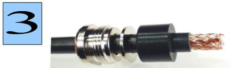
Remove 8 mm of the outer sheath with a knife.
