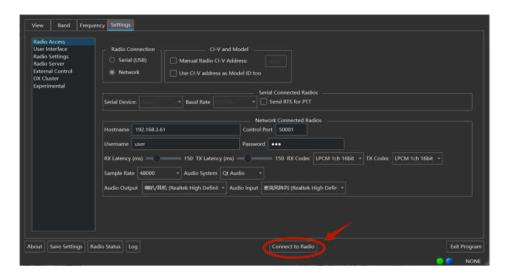
4. After connecting, a signal will appear in the spectrum display window of the main interface "View", indicating that the X6100 has established a correct connection with the computer.
