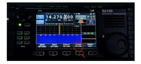
② After entering the system settings, open the WFSERVER settings interface (use the MFK knob to select WFSERVER, then short press to confirm).
