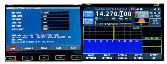
2. To use WiFi wireless connection, you also need to enter the radio station WLAN settings function and configure the radio IP server address:
