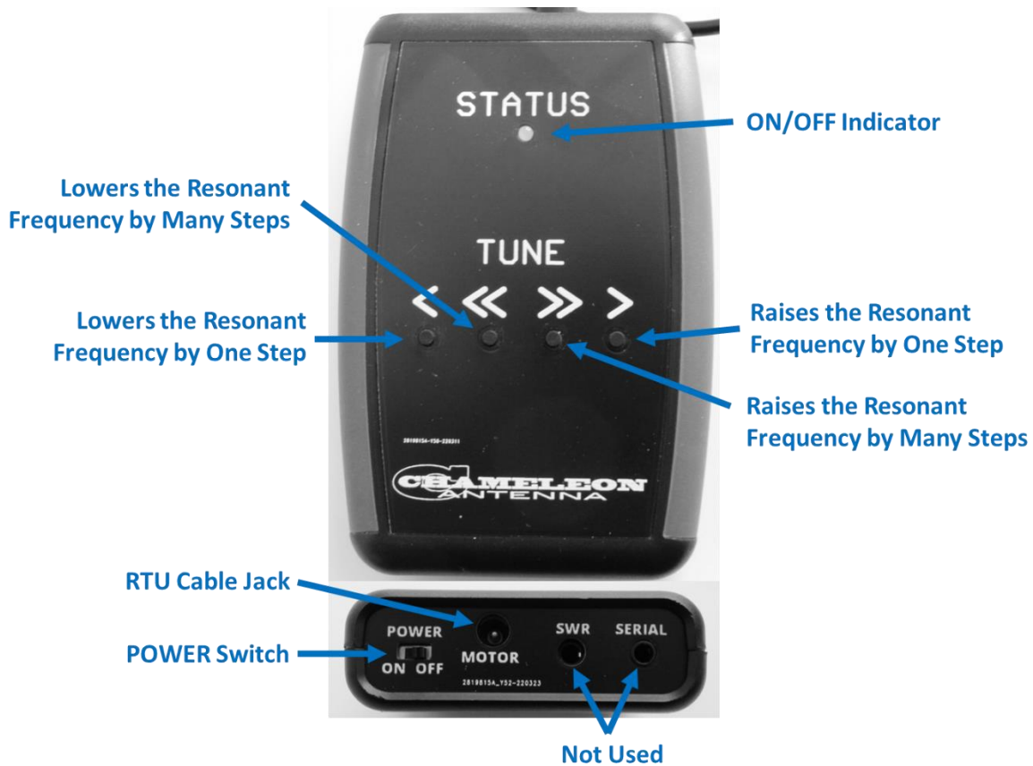
Plate 9. Remote Tuner Unit Controls and Connections Location.
