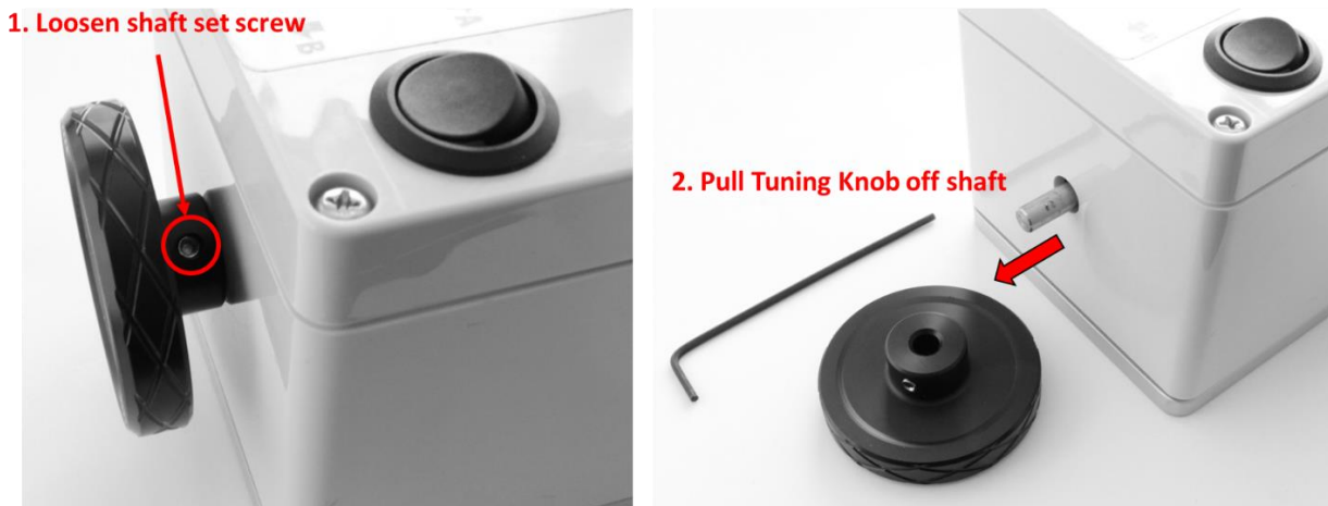
Plate 2. Tuning Knob Removal.
