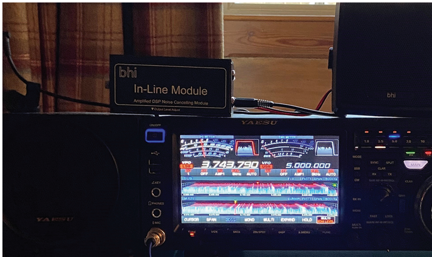
PHOTO 2: The unit in action on top of the author's Yaesu FTDX101MP on 3.743MHz.
