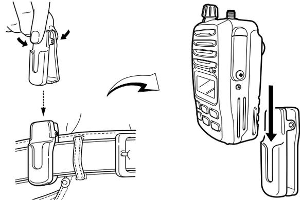
③ Once the transceiver is locked in place, it will swivel 360 degrees.
