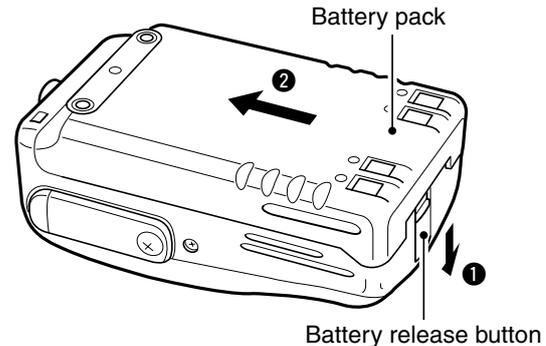
**CAUTION!** When pushing the battery release button, slide the battery pack slightly in the direction of the arrow (2) to ease release. This will prevent possible injuring to your fingers or nails
